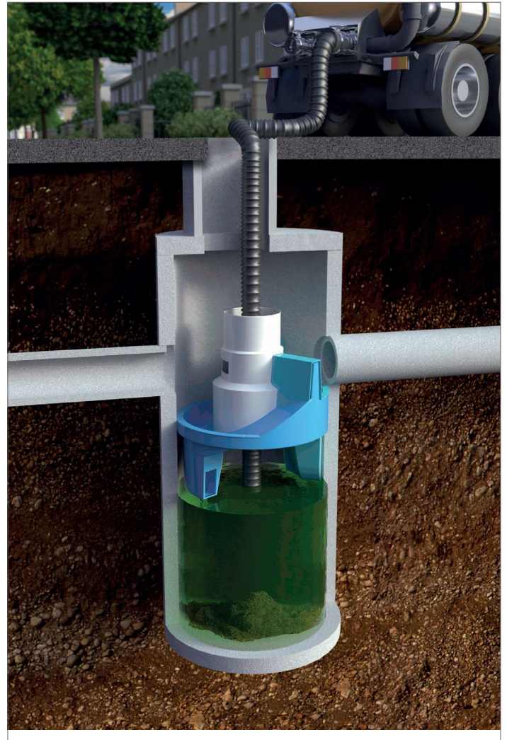
Fig.4 Floatables are removed with a vactor hose
