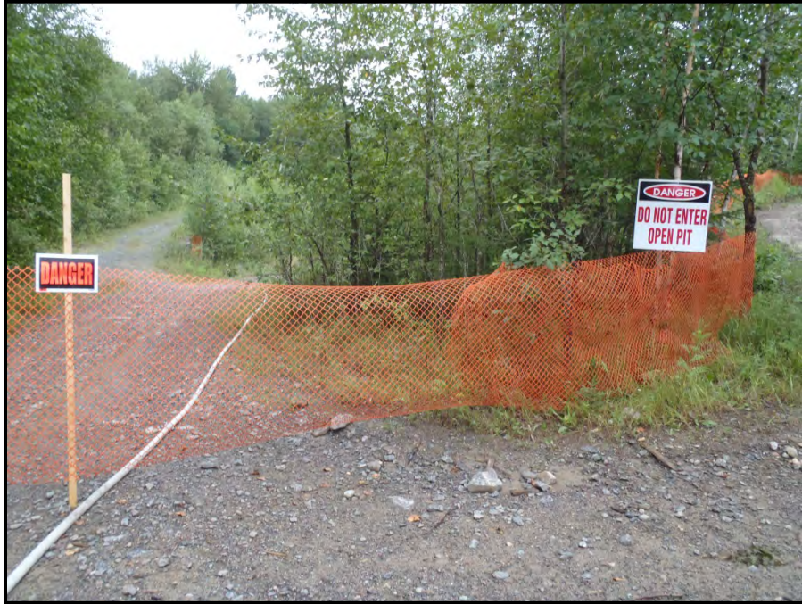
Photo 5: Example of a barrier fence around a pit.
