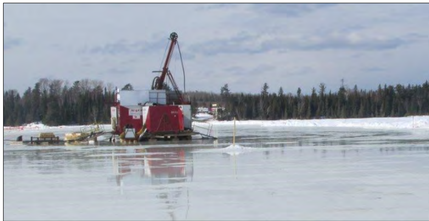
Photo 13: Diamond-drill rig on ice during the winter.
