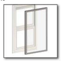
Interior (indoor-mounted) window panels are always fully deployed. They are considered to be tightly attached to the baseline window with no gaps around the edges. Gap of 1 in. between the prime glass and the interior window panel is considered for all qualities.
