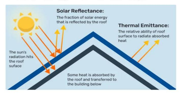
Any roofing system that reduces the energy consumption of the structure beneath can count as a form of energy-efficient roof.
