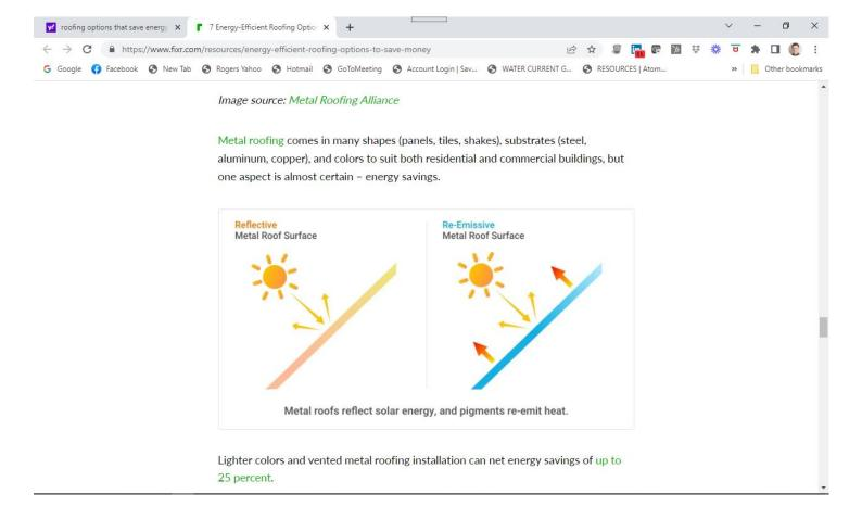
Lighter colors and vented metal roofing installation can net energy savings of up to 25 percent.
