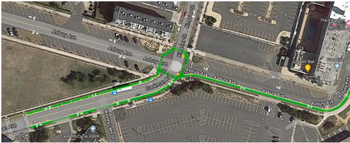
Fig. 1. Temporary bicycle lane. Note that we were unable to paint the entire width of the bicycle lanes in green. Paint was merely used to stripe the lanes.
